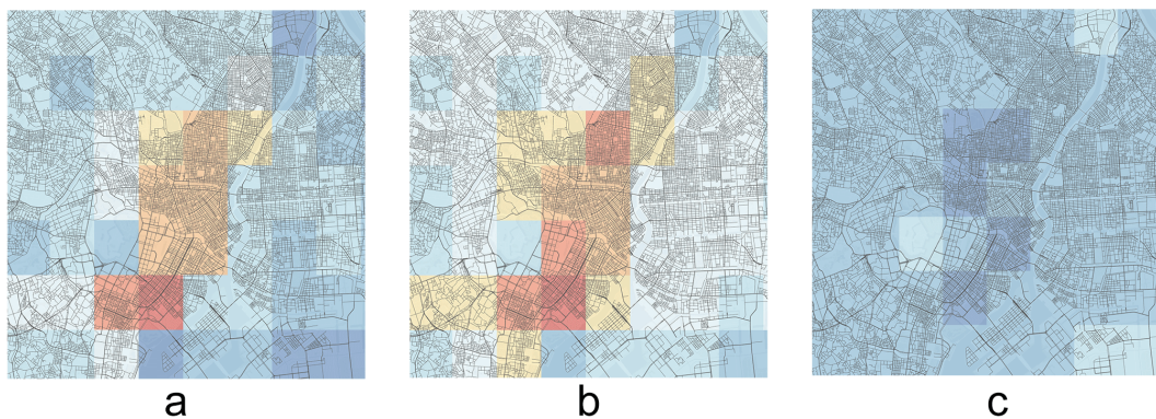
Figure 1: Measures of the a) number of intersections, b) total road length, c) mean road length on subnetwork grids reveal consistent patterns in the road structure that create varying neighborhood ambiances (selected area of central Tokyo shown).
